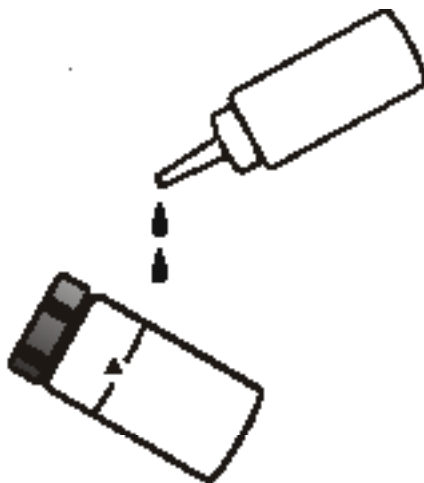
Figure 10 Applying the Silicon Oil
