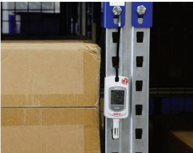
Fig. 5 und 6: The EBI 25-TH temperature data logger with wireless technology, for example, combines the very good measuring accuracy of \pm 0.5K ( -20\text{ }^{\circ}\text{C} ... +40\text{ }^{\circ}\text{C} ) and functionality of a data logger with the possibility of monitoring up to 48 loggers via one interface. With the FDA compliant software Winlog.web it is possible to visualize all measured values live on one screen. In addition, the alarm function guarantees the possibility of a quick reaction in case of temperature or humidity deviations.
