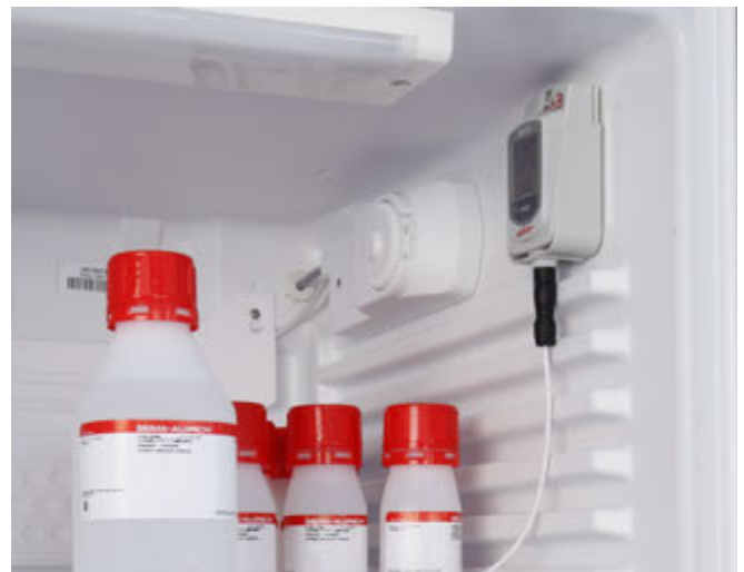
Fig. 5 und 6: The EBI 25-TH temperature data logger with wireless technology, for example, combines the very good measuring accuracy of \pm 0.5K ( -20\text{ }^{\circ}\text{C} ... +40\text{ }^{\circ}\text{C} ) and functionality of a data logger with the possibility of monitoring up to 48 loggers via one interface. With the FDA compliant software Winlog.web it is possible to visualize all measured values live on one screen. In addition, the alarm function guarantees the possibility of a quick reaction in case of temperature or humidity deviations.
