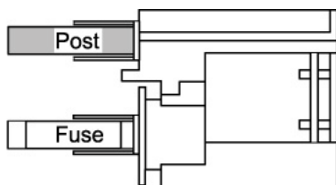
Fuse drawer for 100/120 voltage selection
