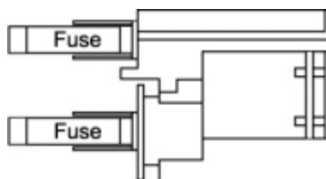
Fuse drawer for 220/240 voltage selection
