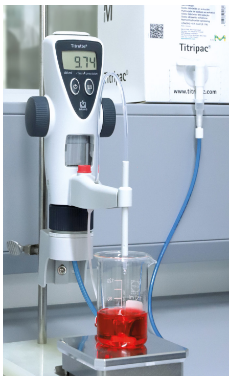
Titrette® extraction system for Bag-in-Box packaging system
