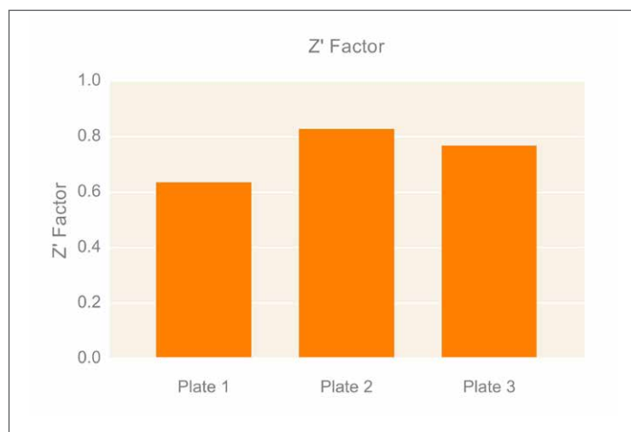
Figure 3. Z' factor. Z' factor calculated from comparing swelling of MDCK cysts exposed to forskolin or media control. N = 16 wells per plate from 3 independent studies.
