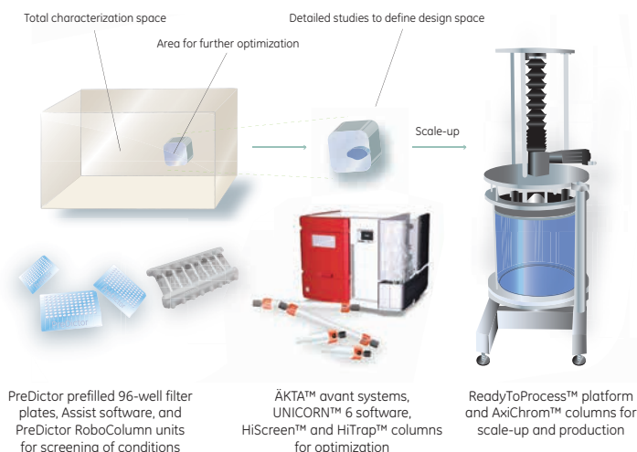
Fig 2. Conceptual visualization of a workflow for process development. Parallel screening by using PreDictor plates or PreDictor RoboColumn units makes it possible to explore a large experimental space for optimal conditions (left). Once these have been identified, fine-tuning and verification are carried out on columns and ÄKTA systems (middle). Finally, scale-up is done under conditions in which a robust production scale process can be operated (right).
