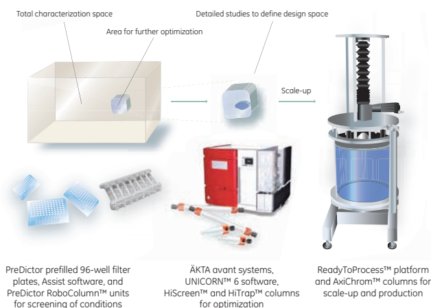
Fig 2. Conceptual visualization of a workflow for process development. Parallel screening using PreDictor plates or PreDictor RoboColumn units makes it possible to explore a large experimental space for best conditions (left). Once these have been identified, fine-tuning and verification are carried out on columns and ÄKTA systems (middle). Finally, scale-up is done under conditions in which a robust production scale process can be operated (right).
