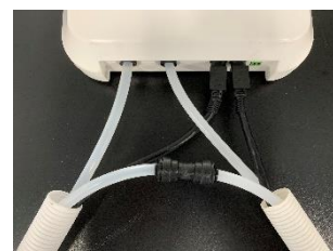
Connection of multiple dispensers for UP water
