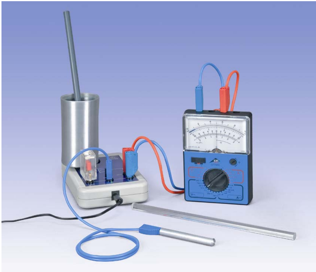
Fig. 1 Experiment set-up for measuring charges in electrostatics
