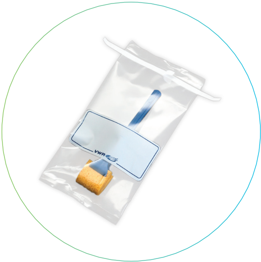
FIGURE 3: Surface sampling sponge with handle.
