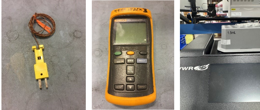
Images left to right: Omega temperature probe, Fluke digital thermometer, 1.5mL Accessory Block
