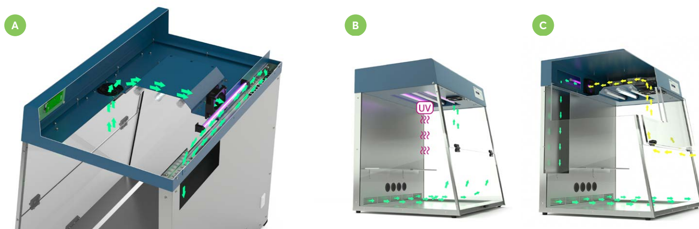
FIGURE 6: Visualization of the air flows inside the PCR workstation with UV air recirculatory (green arrows); A) cross section through the hood; B) workstation in decontamination mode (door is closed); C) workstation in operation mode, yellow arrows display contaminated air from the outside (door is open)
