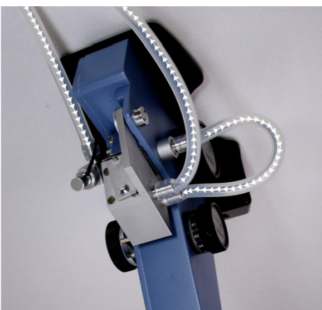
Temperature control from a circulator
