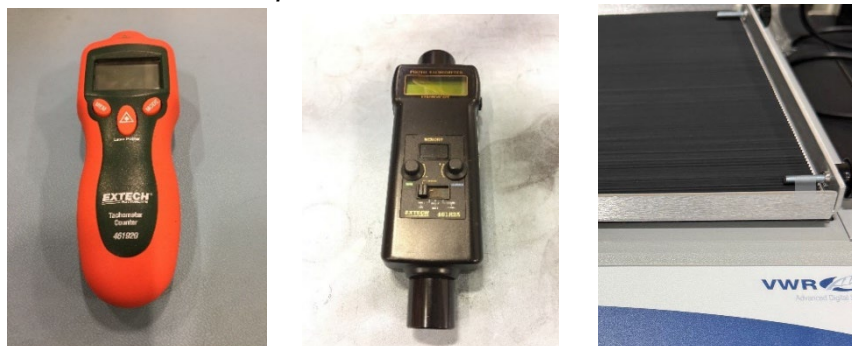
Images left to right: Extech Tachometer, reflective tape, Location of the tape.
