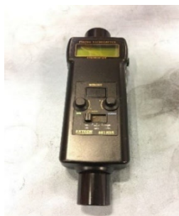
Images left to right: Extech Tachometer, reflective tape, Location of the tape.
