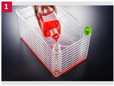
1 Pour the media directly into the Cell Chamber System
