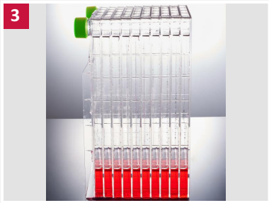
3 Turn 90° so the filling inlet is upward, the medium will be separated, with equal amounts in each chamber
