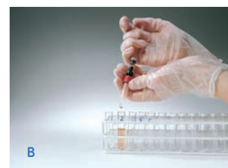
Fig 2. Using a HiTrap column with a syringe. A Prepare buffers and sample. Remove the column's top cap and snap off the end. B Load the sample and begin collecting fractions. C Wash, elute, and continue collecting fractions.
