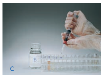
Fig 2. Using a HiTrap column with a syringe. A Prepare buffers and sample. Remove the column's top cap and snap off the end. B Load the sample and begin collecting fractions. C Wash, elute, and continue collecting fractions.
