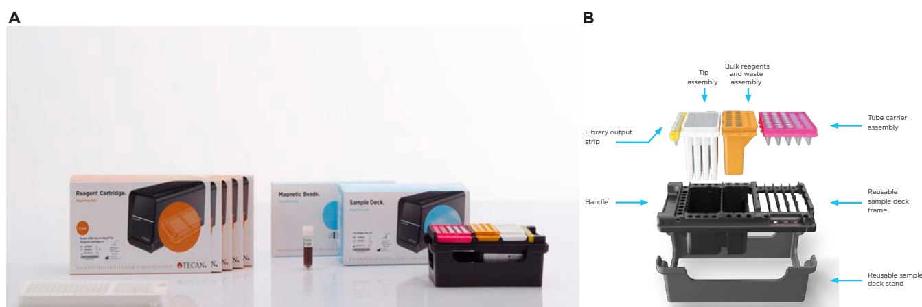
Figure 2: Components of a MagicPrep NGS kit. The kits supplied for the MagicPrep NGS system provide everything necessary for a run. A) Each MagicPrep NGS kit comes with magnetic beads (not shown), reagent cartridges and sample deck consumables. These consumables provide all the reagents, adaptors, buffers, bead, and tips needed for library prep. B) Sample deck consumables are inserted into the sample deck frame to assemble the final sample deck. After adding the samples and beads, the assembled sample deck is ready to be inserted into the MagicPrep NGS system to start a run.
