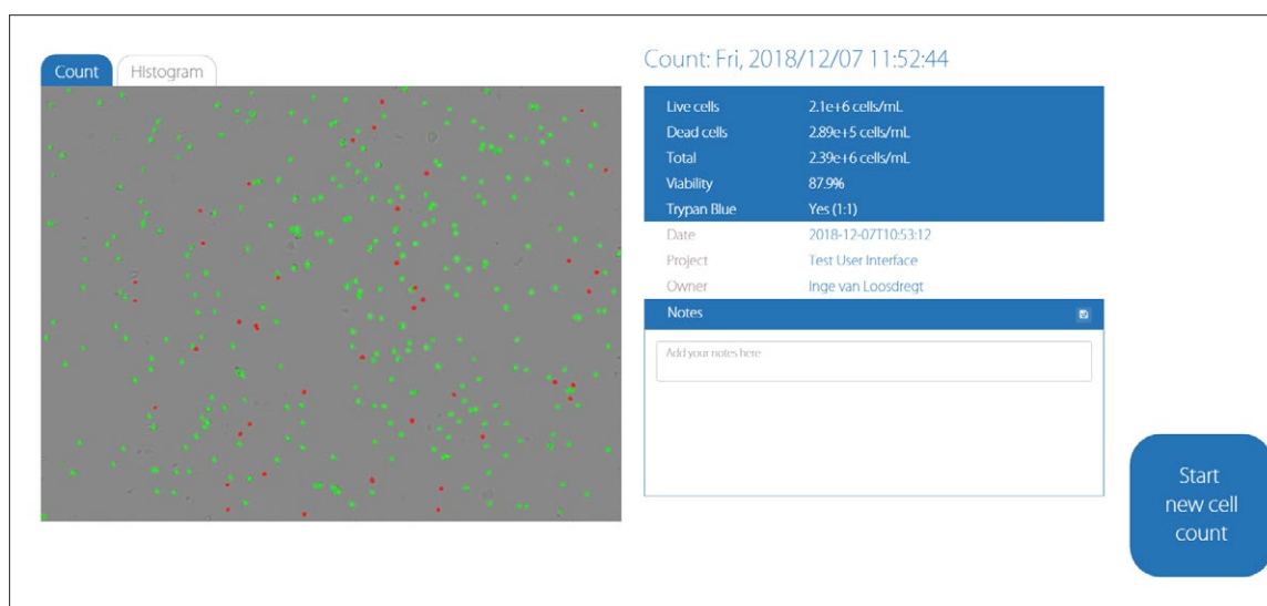
Figure 4. New results page. Click on the “Histogram” tab to view the histogram of the diameter of live and dead cells. The Trypan blue dilution is displayed in the results box.
