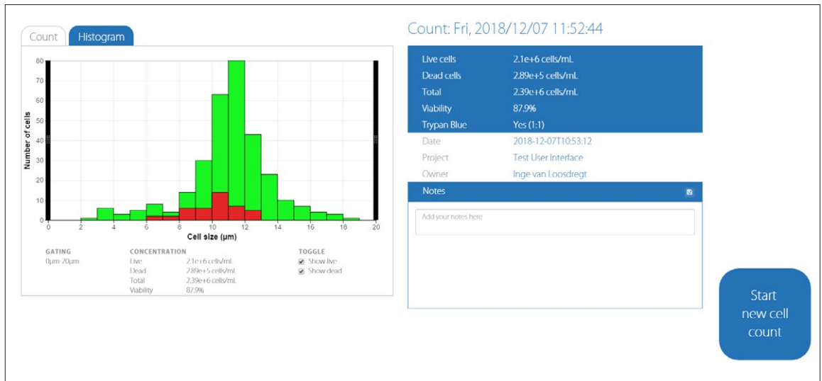
Figure 5. The size histograms of the live and dead cells are displayed in one chart. The histograms can be gated by moving the black bars on the left and right side of the chart.
