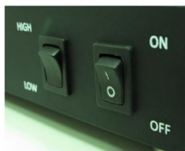
FRONT OF THE VWR® BLUE TRANSILLUMINATOR- POWER ON/OFF AND ADJUSTING INTENSITY
