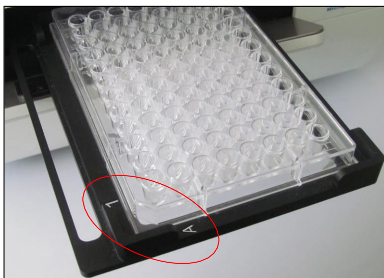
Fig. 10 Placement of a plate on the plate platform
