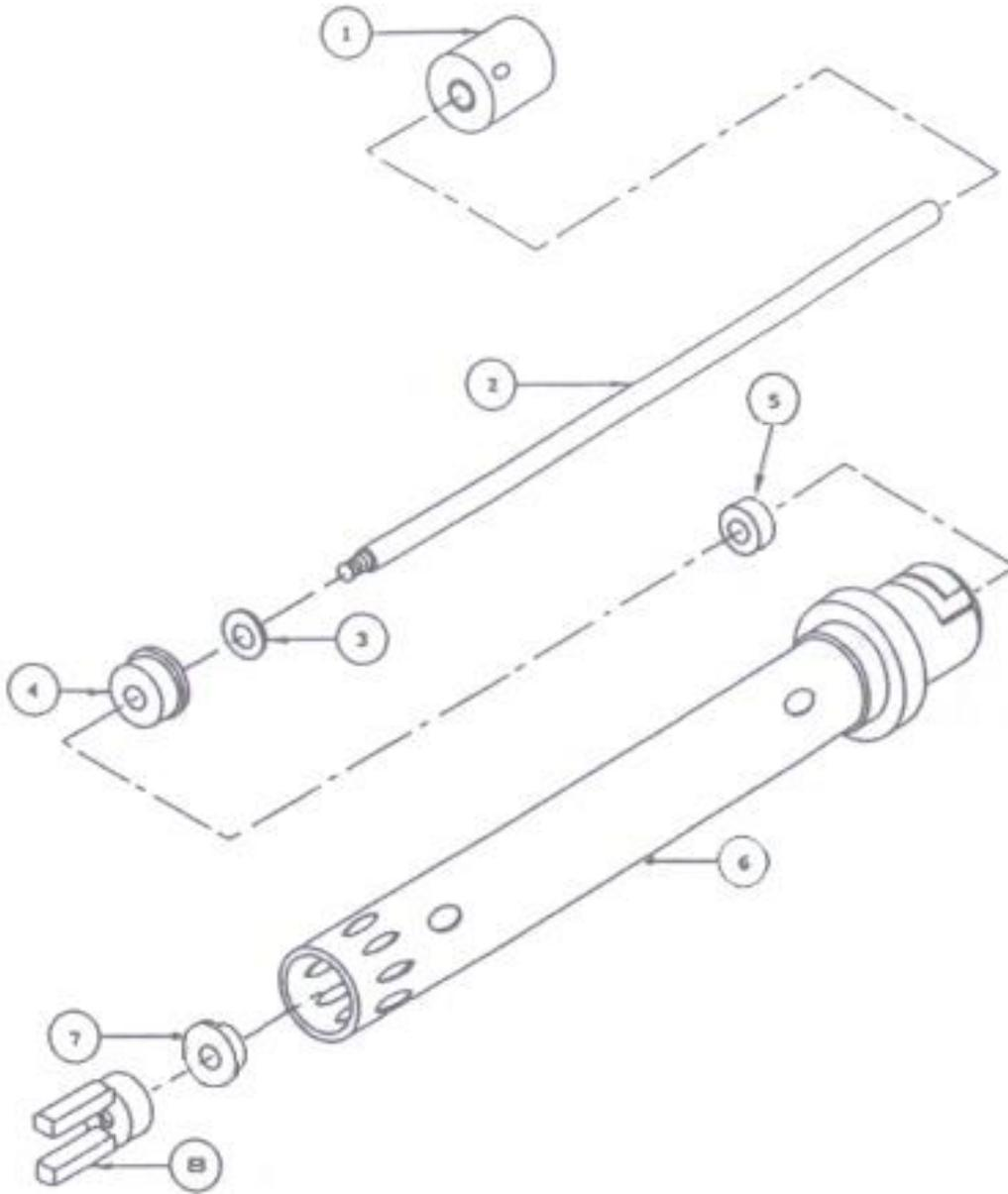
**Generator Probe Replacement Parts**
