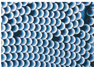
Fig. 32. Electron micrograph of MonoBeads showing their distinct monodispersity
