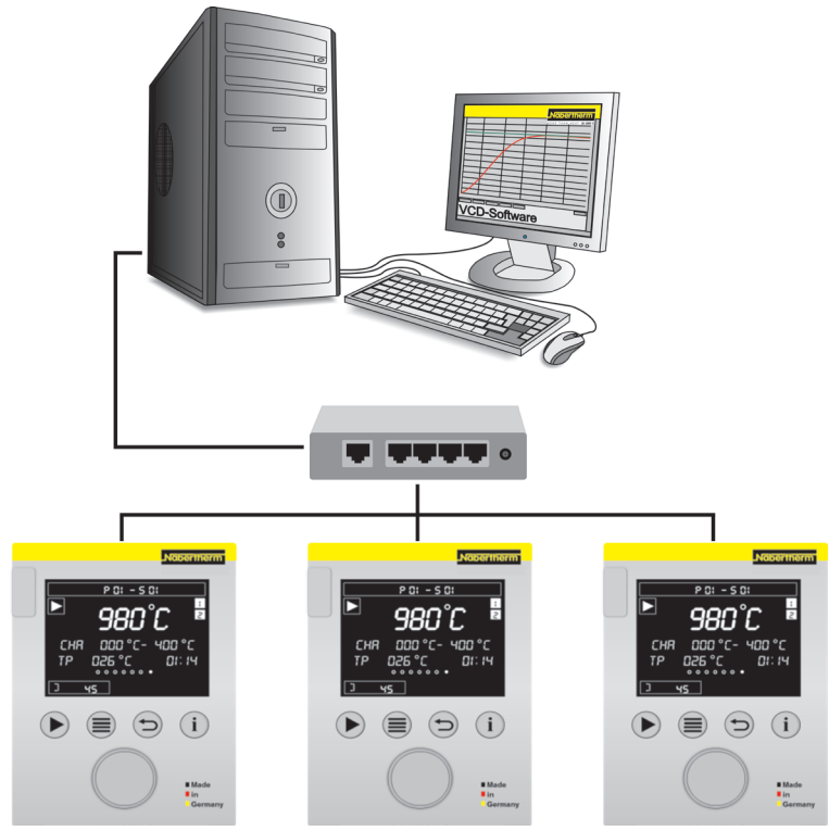
Example lay-out with 3 furnaces
