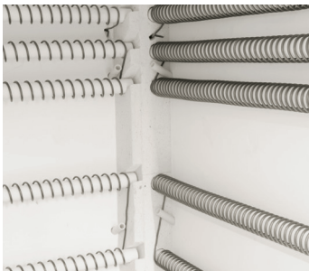
LF furnace design provides for shorter heating and cooling times
