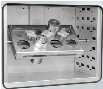
Electrical rotating device as additional equipment
