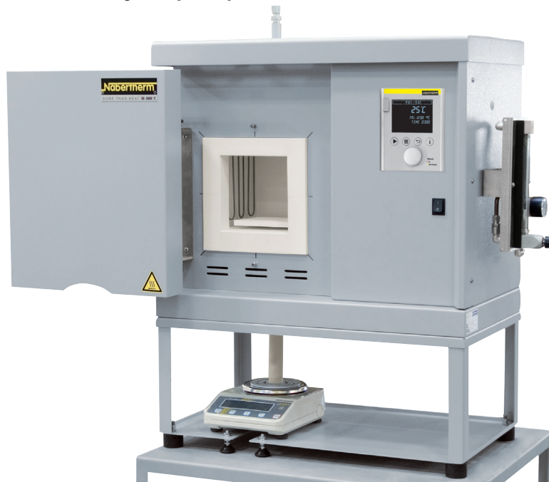
High-temperature furnace LHT 04/16 SW with scale for measuring weight reduction during annealing and with gas supply system
