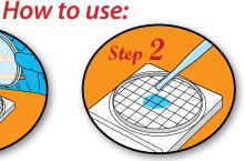
Drop 1ml of specimen (dilute if necessary) in the middle of dry sheet.
