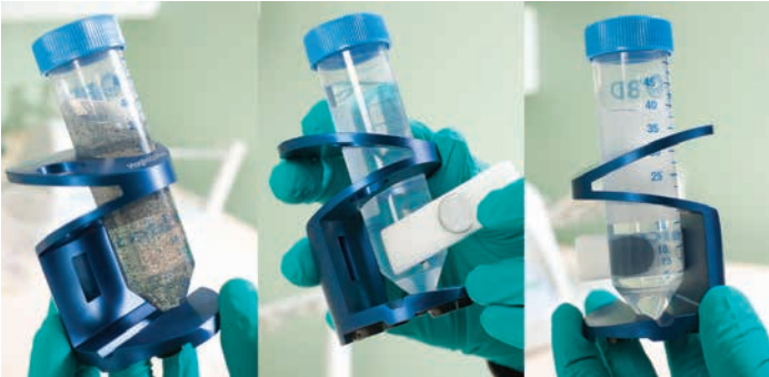
Fig 3.9. (A) MagRack 6 and (B) MagRack Maxi magnetic racks consist of an aluminum housing with a detachable magnetic bar. When the magnetic bar is inserted (center images), the high-density magnetic beads become attracted to the magnet in seconds. This allows easy removal of supernatant while the magnetic beads remain in the tube (images on the right).
