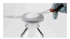
Place base on the receiving vessel with gasket seal seated on the rim of the vessel.\* Place the membrane on the clean, dry filter support. If using wwPTFE turn on vacuum to remove potential curling and seat the filter disc.
