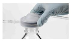
\* Always use a safety-coated receiving vessel that is less than 4 L and rated for vacuum applications. Failure to do so may result in implosion of the receiving vessel and potential injury to the user.
