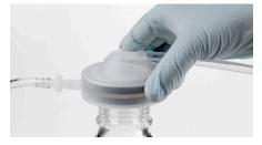
While holding filter housing assembly on receiving vessel, attach vacuum tubing from vacuum source to the vacuum port adaptor located on the side of the housing base.
