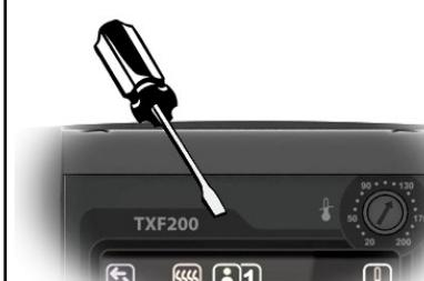
Rotate dial to desired temp cut-out (above set point)
