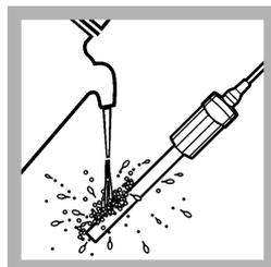
**4.** Rinse the probe with deionized water. Dry with a no-lint cloth.
