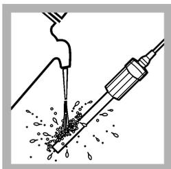
3. Rinse the probe with deionized water and then with the sample. Dry with a no-lint cloth.
