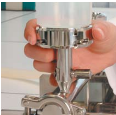
Fig 2. Pre-sterilized funnel is installed on filter base over membrane.
