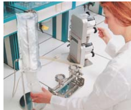
Fig 1. By taking a new pre-sterilized funnel, a membrane is dispensed automatically. (Workflow continued on next page)
