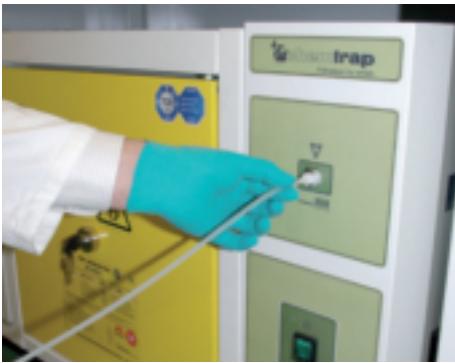
Connect one end of the silicone tube to the sampling port located on the control panel
