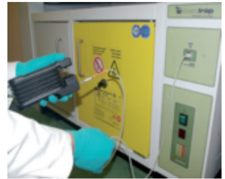
Take a sample of air by activating the pump. To find the number of strokes, refer to the instructions supplied with the tubes used.
