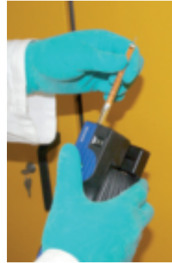
Connect the broken tube to the pump taking care to check that it is inserted in the right direction. The colorimetric tubes are marked.
