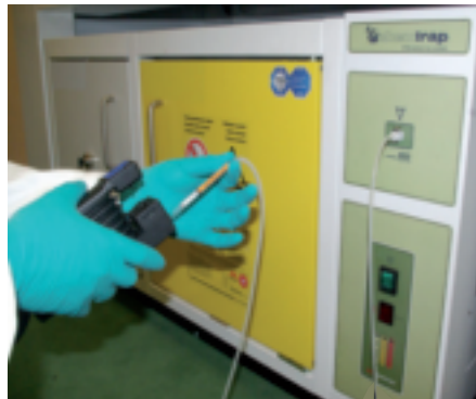
Connect the flexible silicone tube to the other end of the broken tube
