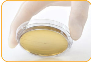
2. Gently press plate to surface without twisting or sliding.
