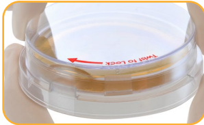
3. Twist clockwise until frosted bands line up and lid locks into place. Incubate at 30 °C - 35 °C. After 48 - 72 hours, count the number of colonies. Record your results.
