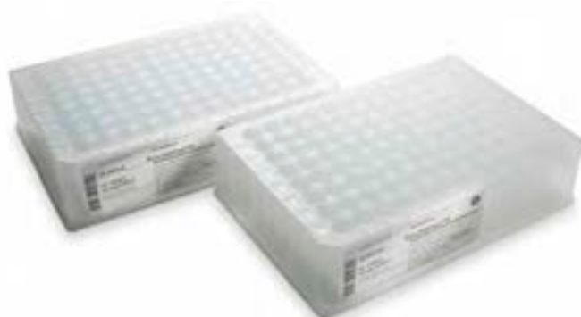
Fig 3.6. His MultiTrap HP and His MultiTrap FF are prepacked 96-well filter plates for high-throughput expression screening of histidine-tagged proteins.
