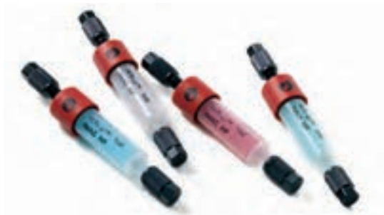
Fig 3.49. HiTrap IMAC HP 1 ml columns charged with \text{Cu}^{2+} , \text{Zn}^{2+} , \text{Co}^{2+} and \text{Ni}^{2+} , respectively.
