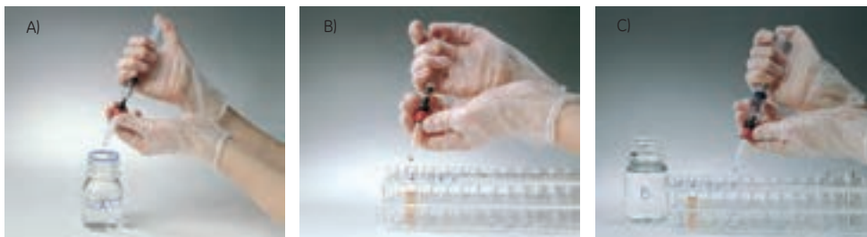
Fig 5.10. Using a GSTrap column with a syringe. A) Prepare buffers and sample. Remove the column's top cap and snap off the end. B) Load the sample and begin collecting fractions. C) Wash and elute, continuing to collect fractions.
