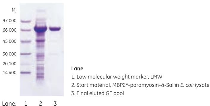
Fig 6.4. SDS-PAGE analysis (reducing conditions) of the purification of MBP2*-paramyosin- \delta -Sal.
