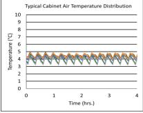
Performance data acquired at 22°C ambient, 4°C nominal set point in an empty cabinet with drawers using air probes, during stabilized steady state operation and a DAQ sampling rate of one measurement every 10 seconds
