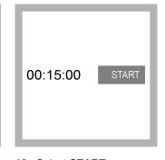
**12.** Select **START**. If the sample temperature is less than 10 °C (50 °F), wait 20 minutes instead of 15 minutes.
