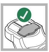
**2.** Keep the sample port cover closed during startup.
