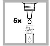
**9.** Immediately add **5** drops of Fluorescence Sulfite **Reagent 2**. Hold the bottle vertically.
