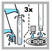
**6.** Rinse the sample vial and cap three times with the sample.
