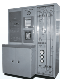
Model KLA-2 Column (40 μm particles) Analysis time: 22 hrs
