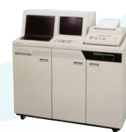
Model L-8500 Column (3 μm particles) Nihydryn two-reagent system Analysis time: 30 min
