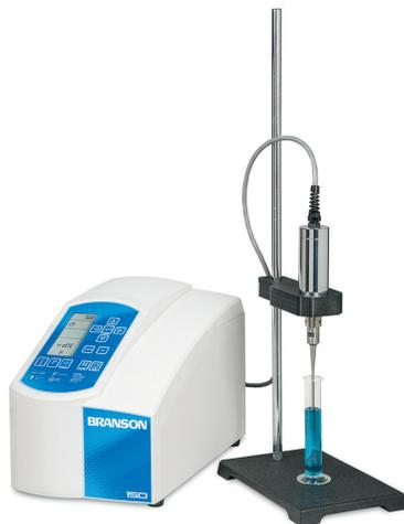
**Stand and Converter Holder:** The support stand with stainless steel rod accommodates Branson's 20 kHz converter. The converter holder supports the ultrasonic stack (converter and horn) and is adjusted easily to properly position the horn in the sample.
