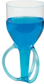
**Rosette Cell:** Branson's Rosette Cell provides a unique flow pattern of substances for exposure to ultrasonic energy during circulation through the cell. When it is immersed in a cooling bath, the enlarged glass surface area and circulation through the side arms provide an efficient means of heat exchange.
