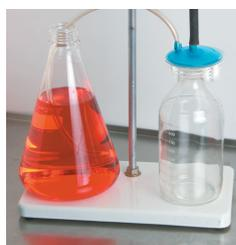
2. Connect the vacuum tubing to the port marked "VACUUM" on the VacuCap device. Refer to product insert for safety precautions.
