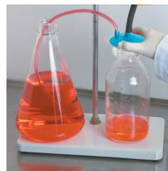
3. While holding the VacuCap device securely on the filtrate container, start the vacuum. The VacuCap device will seal securely to the container top and fluid will be drawn.
