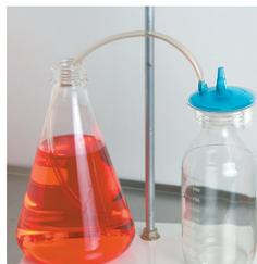
1. Connect the feed tubing to the port marked "INLET" on the VacuCap device. Place the opposite end of the tubing in the unfiltered fluid to be drawn.
