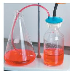
4. When filtration is complete, switch off the vacuum pump allowing the vacuum inside the receiving container to dissipate. Refer to the product insert for complete instructions.
