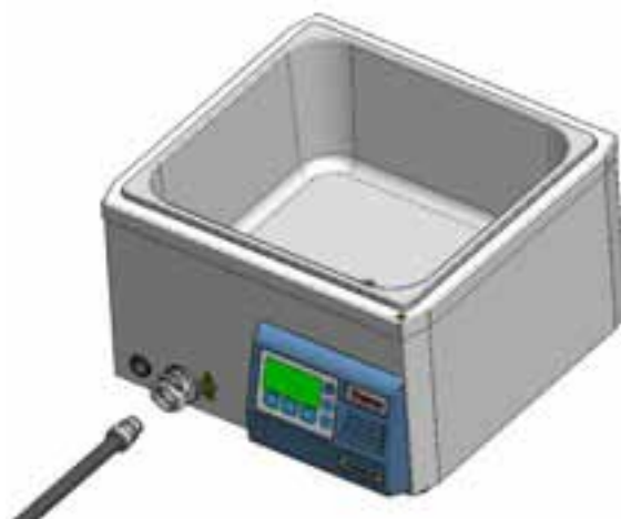
Figure 3-3– GP Bath Drain Hose
