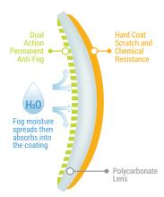
HexArmor® TruShield®S dual-coated lenses are ideal for environments where there's a high degree of dirt or debris, coupled with more severe fogging factors.
