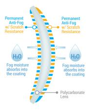
Dual-coated lenses are ideal for clean to moderately dirty work environments, where workers transition from cold to hot or hot to cold.
