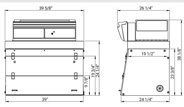
Please add 5 7/8" between the last filter and the ceiling to allow good air recirculation and to replace filters easily.
