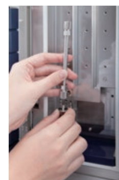
A view of operation of attaching a column
