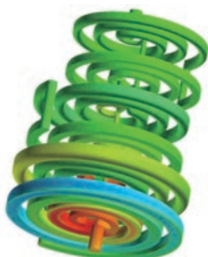
Double corkscrew mixer flow path diagram
