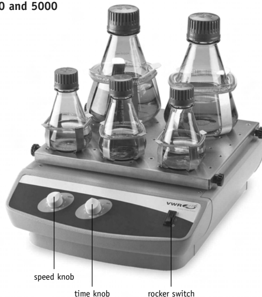
Standard Orbital Shaker with optional platform and flask clamps
