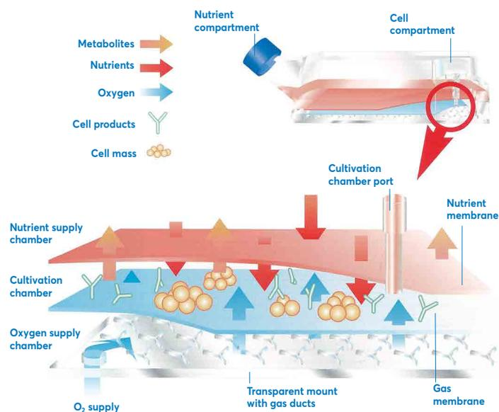
The Corning CELLine disposable bioreactor is a two-chamber cell cultivation vessel in which the chambers are separated by a 10 kD molecular weight cut-off membrane. This arrangement allows for high density cell culture and high-yield monoclonal antibody (mAb) production while maintaining a concentrated product.
