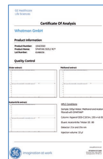
Fig 1: SPARTAN syringe filters are tested and certified for the absence of UV-absorbing substances at wavelengths of 210 and 254 nm with water, methanol, and acetonitrile.
