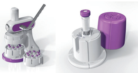
Fig 6: Left: Multi-unit compressor holding eight Mini-UniPrep G2 filters. Right: Single Mini-UniPrep G2 filter in a hand compressor. The compressors shown are for illustration purposes only and are not intended to represent the actual compressors. It is the buyer's responsibility to clarify with the seller the exact design of the compressors.
