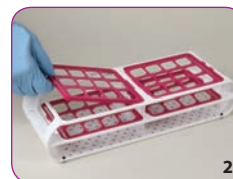
2: Lift out the grid
