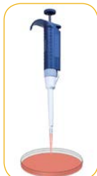
Aspirate sample into 1000µl tip
