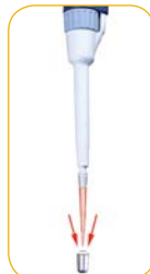
Press FLOWMI onto pipette tip
