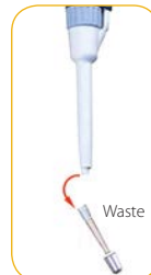
Eject to dispose of tip and FLOWMI
