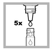
8. Immediately add 5 drops of Fluorescence Total Chlorine Reagent 1. Hold the bottle vertically.
