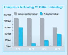
Up to 90 % less energy consumption at 22 °C ambient temperature
