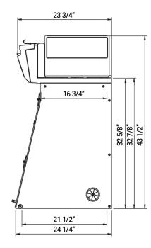
Please add 5 7/8" between the last filter and the ceiling to allow good air recirculation and to replace filters easily.
