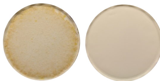
Figure 3. Pictures of the CN membrane treated with tap water (left) and treated with ultrapure water produced from the GenPure Pro system fed with tap water (right)
