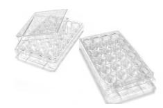
24-Well Plates are available non-sterile, sterile, and treated for tissue culture. Sterile and treated polystyrene plates are gamma-irradiated for sterility and are individually packed with lids.
